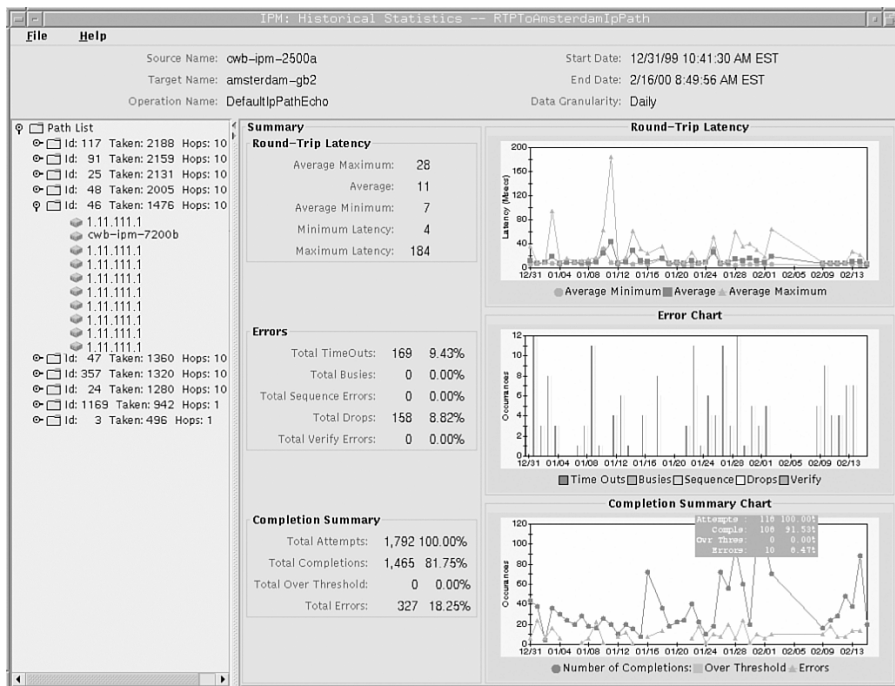
Figure 2-6 Sample Screen of a Management Application with Performance Graphs (Cisco Works IP Performance Monitor)
