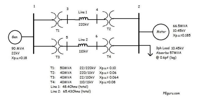
4. Make the admittance matrix, Ybus, for the following network. Given parameters are impedance in per-unit.
