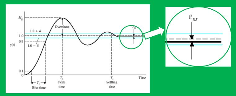
Steady State Error  $(e_{ss})$ : The difference b/w the steady state output value and the reference input value at steady state
