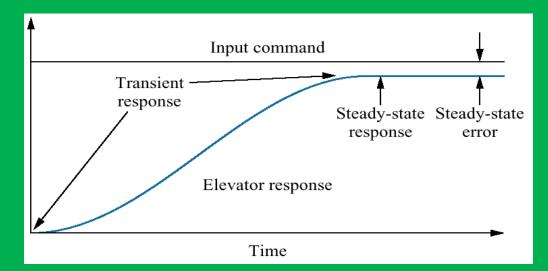
A distinct advantage of f/back control system is the ability to adjust transient and steady-state response
