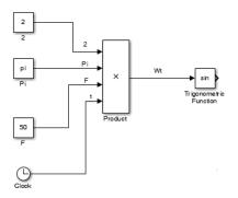
Now our desired equation is  $V_m Sin \omega t$  it means that  $V_m$  is in product with the Sin $\omega t$  so multiply them we get.
