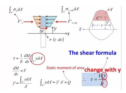
Example 1: For the rectangular cross-sectional area subjected to internal shear force V, determine the shear stress distribution as a function of y.
