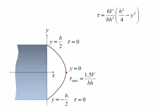
Example 2: For the over hanging beam with the shown loadings and cross section, determine the absolute maximum **shear** stress in the beam, and stretch the shear stress distribution.
