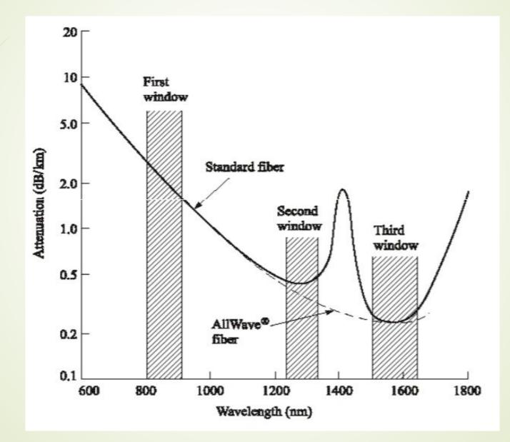
Attenuation is wavelength dependent, hence proper selection of operating wavelength is required.
