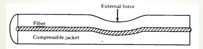
A compressible jacket extruded over a fiber reduces micro bending resulting from external forces.
