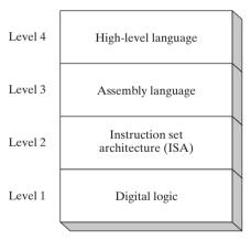
Figure 1–1 Virtual machine levels.
