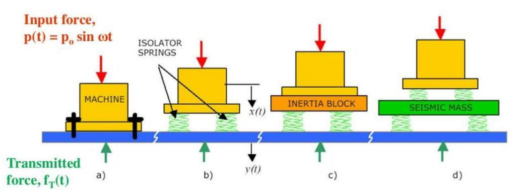
Vibration isolation systems: a) Machine bolted to a rigid foundation b) Supported on isolation springs, rigid foundation c) machine attached to an inertial block d) Supported on isolation springs, non-rigid foundation (such as a floor); or machine on isolation springs, seismic mass and second level of isolator springs
