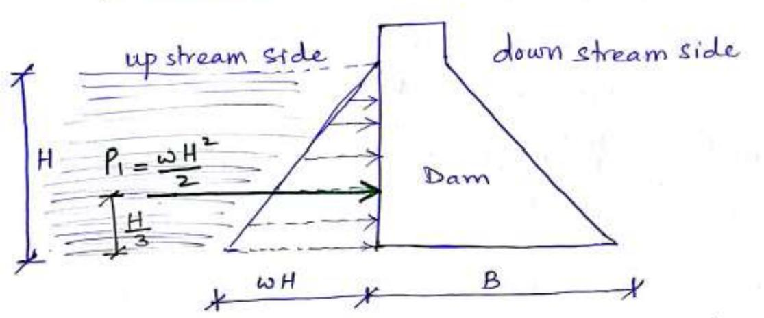
The total pressure is in horizontal direction and acts on the upstream face at a height  $\frac{H}{3}$  from the bottom. The pressure diagram is triangular and the total pressure is given by;  $P_1 = \frac{W}{2} + \frac{H}{3}$
