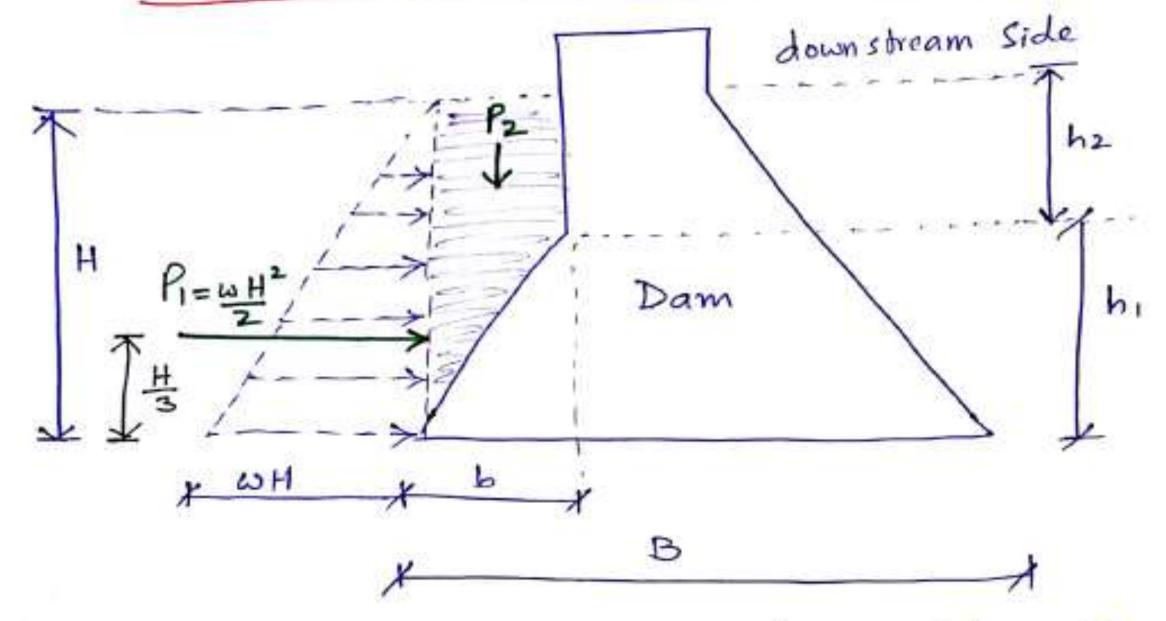
Here in addition to the horizontal water pressure pressure pressure of the previous case, their is vertical pressure of the water.
