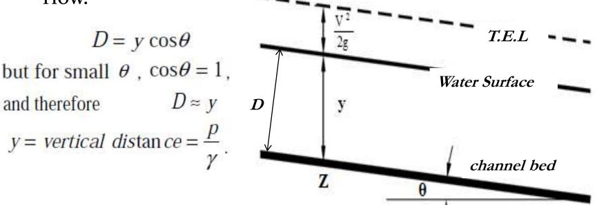
Unless mentioned otherwise, the depth of flow and the depth of flow section will be assumed equal. For uniform flow the depth attains a constant value known as the normal depth, yn
