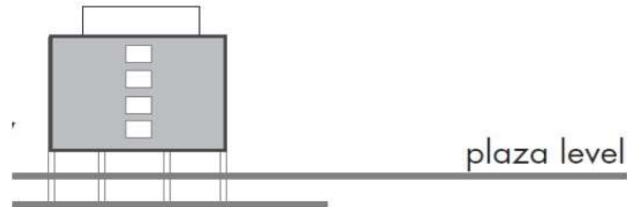
Cross section, Olive View hospital, showing the second-floor plaza and the discontinuous shear wall.
