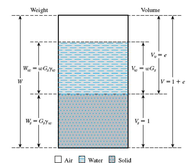
$$\gamma = \frac{W}{V} = \frac{W_s + W_w}{V} = \frac{G_s \gamma_w + w G_s \gamma_w}{1 + e} = \frac{(1 + w) G_s \gamma_w}{1 + e}$$
