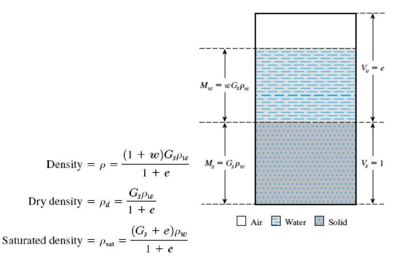
where  $\rho_w = \text{density of water} = 1000 \text{ kg/m}^3$ .
