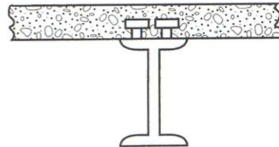
(g) Composite steel-concrete
