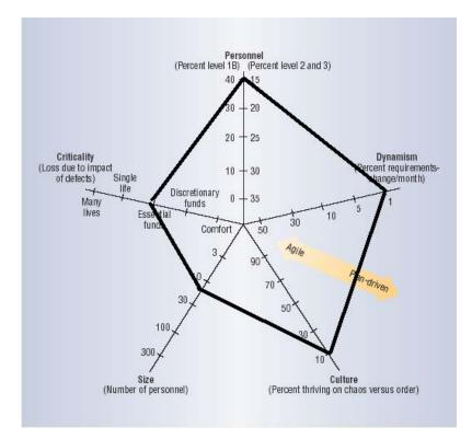
Figure 2: Example Polar Chart. (adapted from (Boehm and Turner, June 2003))
