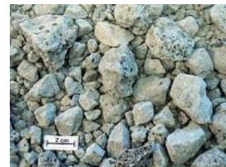
Figure 3. Artificial aggregates example - Air-cooled blast furnace slag (3).
