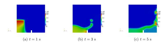
Figure 3: Fluid pressure during breaking of a dam on Jupiter.
