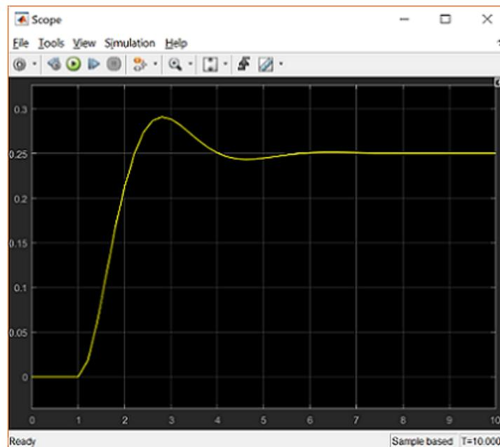
Note that the step response does not begin until  $t = 1$ . This can be changed by double-clicking on the *step* block. Now, we will change the parameters of the system and simulate the system again. Double-click on the *Transfer Function* block in the model window and change the denominator to:
