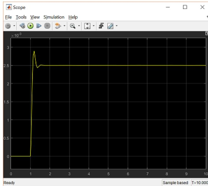
Since the new transfer function has a very fast response, it compressed into a very narrow part of the scope window. This is not really a problem with the scope, but with the simulation itself. Simulink simulated the system for a full ten seconds even though the system had reached steady state shortly after one second.
