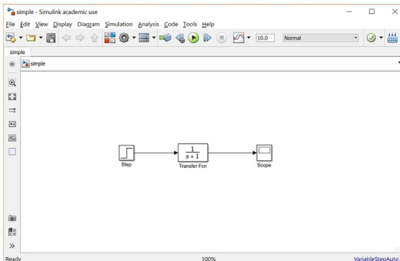
The simple model consists of three blocks: Step, Transfer Function, and Scope.
