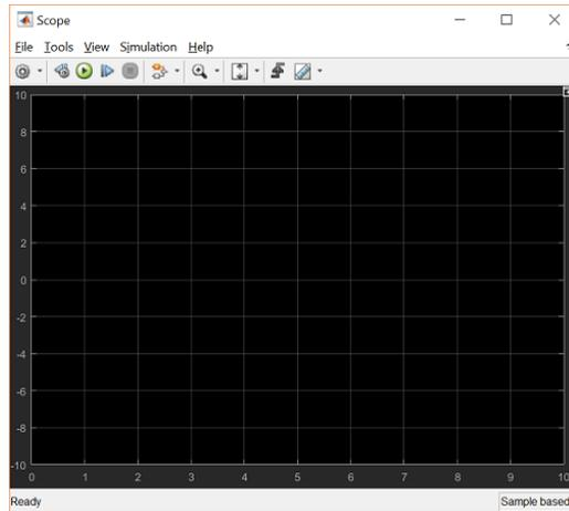
When a simulation is performed, the signal which feeds into the scope will be displayed in this window. Then, to start the simulation, either select **Run** from the **Simulation** menu, click the **Play** button at the top of the screen, or hit **Ctrl-T**.
