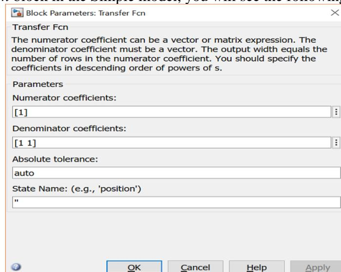
This dialog box contains fields for the numerator and the denominator of the block's transfer function. By entering a vector containing the coefficients of the desired numerator or denominator polynomial, the desired transfer function can be entered. For example, to change the denominator to
