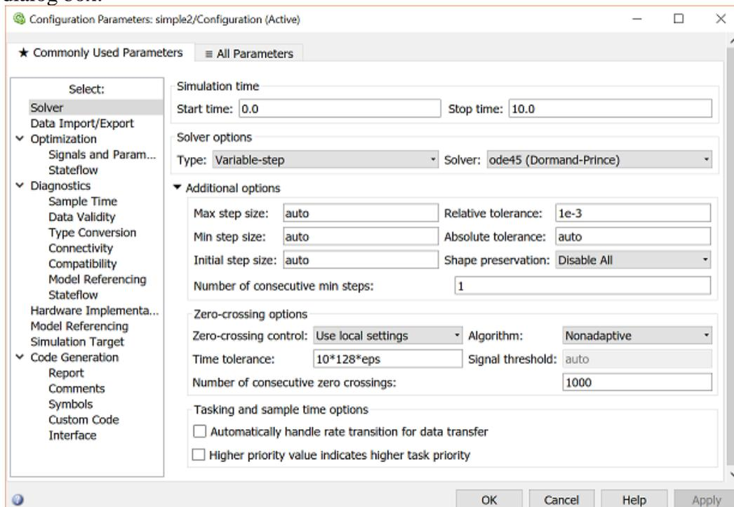
There are many simulation parameter options; we will only be concerned with the start and stop times, which tell Simulink over what time period to perform the simulation. Change **Start time** from 0.0 to 0.8 (since the step doesn't occur until  $t = 1.0$ ).
