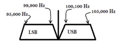
DSB-SC transmission is achieved when carrier is modulated by the modulating signal using balance modulator. When two signals (message and carriers) are fed to the balance modulator, the modulator will produce the amplitude modulated signal with two side bands and carrier is cancelled out.
