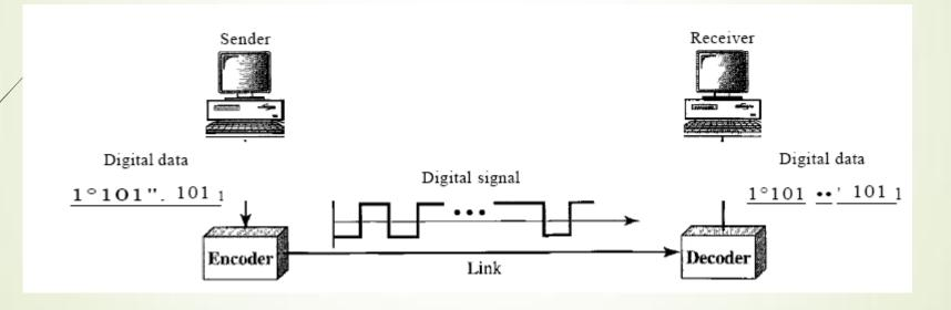
Line coding and decoding
