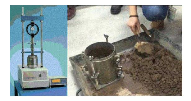
California Bearing Ratio Test on Subgrade Soil
