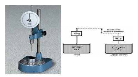
**Determination of Penetration Value of Bitumen**
