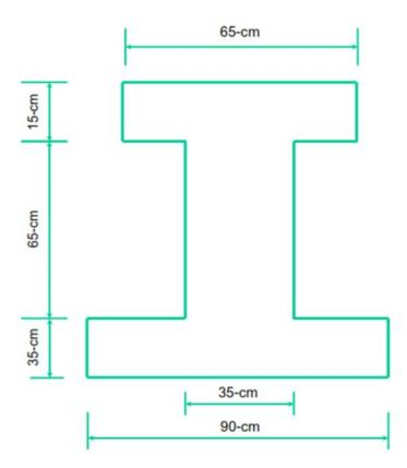
(b) For mid area (65cm x 35cm) only find the moment of inertia, Radius of Gyration & Section moduli. (Marks=2+2+2, CLO-02)
