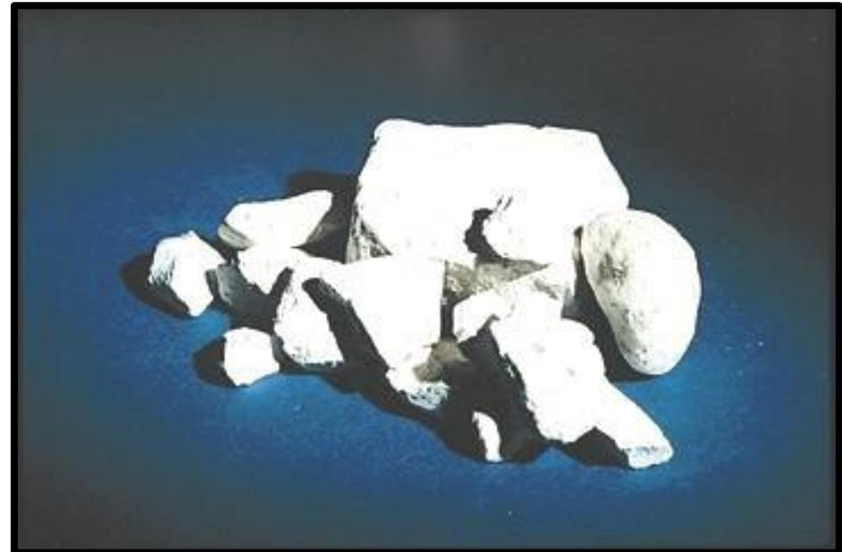
Gypsum, a source of sulfate, is inter-ground with Portland clinker to form Portland cement. It helps control setting, drying shrinkage properties, and strength development
