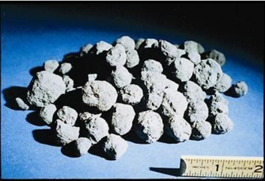
Portland cement clinker is formed by burning calcium and siliceous raw materials in a kiln. This particular clinker is about 3mm to 20 mm (3¼ in.) in diameter
