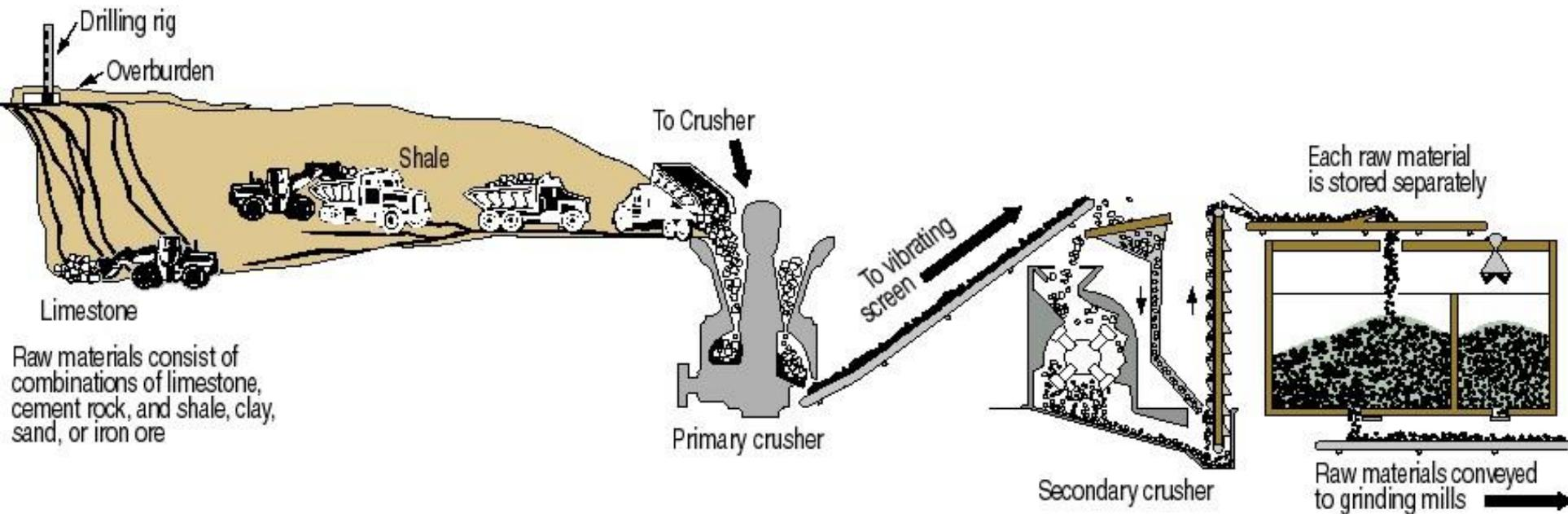
**1. Stone is first reduced to 125 mm (5 in.) size, then to 20 mm (3/4 in.), and stored.**
