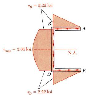
• Determine the shear stress distribution for V = 2.5 kips.
