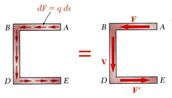
• If the shear load is applied such that the beam does not twist, then the shear stress distribution satisfies
