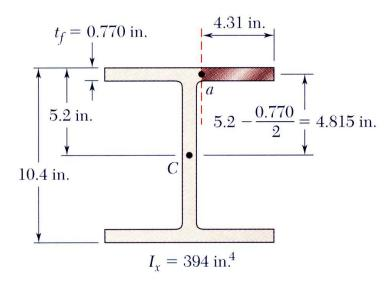
Knowing that the vertical shear is 50 kips in a W10x68 rolled-steel beam, determine the horizontal shearing stress in the top flange at the point *a*.
