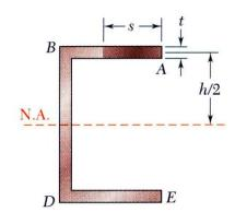
Determine the location for the shear center of the channel section with b = 4 in., h = 6 in., and t = 0.15 in.
