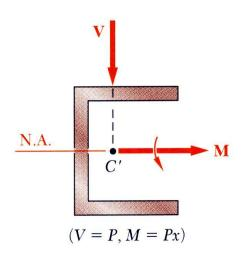
• Beam without a vertical plane of symmetry bends and twists under loading.
