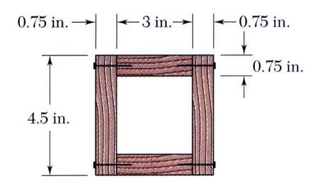
A square box beam is constructed from four planks as shown. Knowing that the spacing between nails is 1.5 in. and the beam is subjected to a vertical shear of magnitude V = 600 lb, determine the shearing force in each nail.
