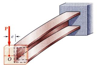
• When the force P is applied at a distance e to the left of the web centerline, the member bends in a vertical plane without twisting.
