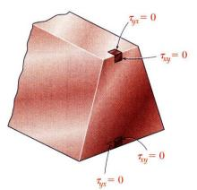
• The *average* shearing stress on the horizontal face of the element is obtained by dividing the shearing force on the element by the area of the face.
