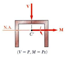
Beam loaded in a vertical plane of symmetry deforms in the symmetry plane without twisting.
