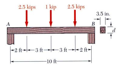
A timber beam is to support the three concentrated loads shown. Knowing that for the grade of timber used,
