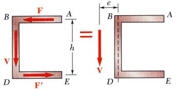
• F and F' indicate a couple Fh and the need for the application of a torque as well as the shear load.
