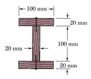
A beam is made of three planks, nailed together. Knowing that the spacing between nails is 25 mm and that the vertical shear in the beam is V = 500 N, determine the shear force in each nail.
