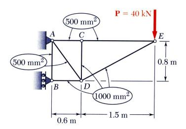
Members of the truss shown consist of sections of aluminum pipe with the cross-sectional areas indicated. Using E = 73 GPa, determine the vertical deflection of the joint C caused by the load P.
