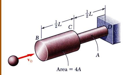
Body of mass m with velocity  $v_0$  hits the end of the nonuniform rod BCD. Knowing that the diameter of the portion BC is twice the diameter of portion CD, determine the maximum value of the normal stress in the rod.
