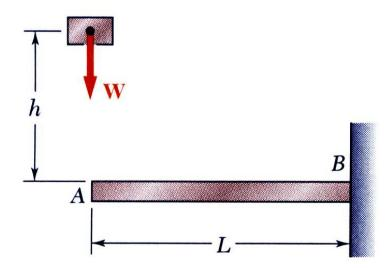
A block of weight W is dropped from a height h onto the free end of the cantilever beam. Determine the maximum value of the stresses in the beam.
