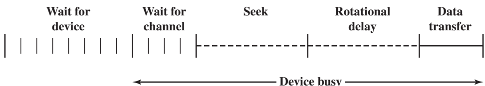
Figure 6.5 Timing of a Disk I/O Transfer
