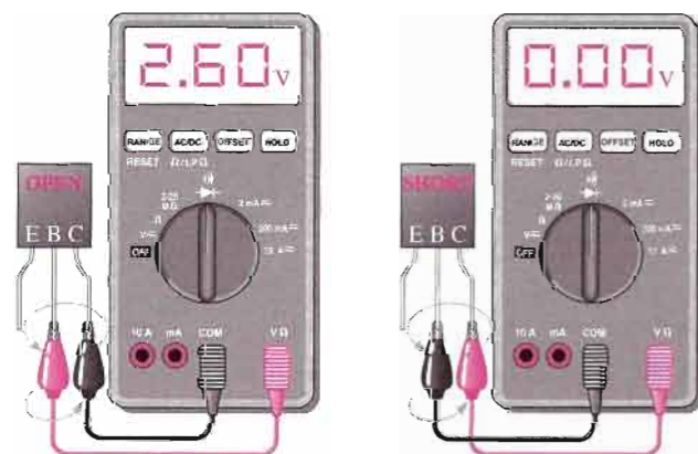
(a) Forward-bias test and reverse-bias test give the same reading (2.60 V is typical) for an open BC junction.
