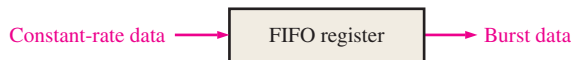
(c) Data input at a constant rate can be stored and then output in bursts.
