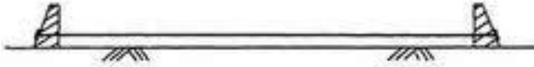
(a) Tendons stressed between abutments
