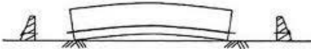
(c) Tendons released and prestress transferred
