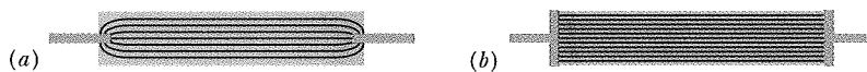
Fig. 26-8 Two ways of applying a potential difference to a conducting rod. The gray connectors are assumed to have negligible resistance. When they are arranged as in (a) in a small region at each rod end, the measured resistance is larger than when they are arranged as in (b) to cover the entire rod end.
