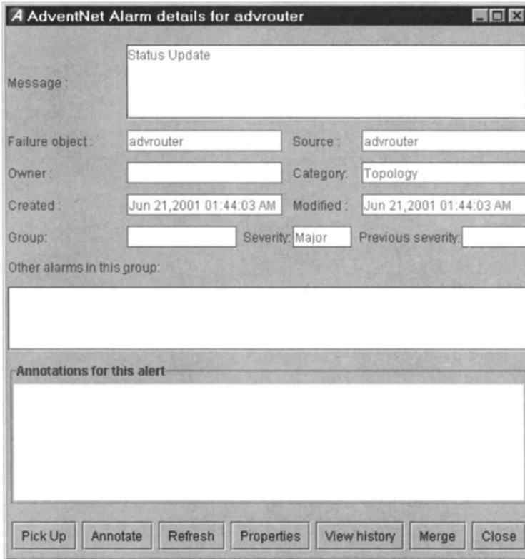
Figure 12.20 Alarm details screen for an object that has experienced failure.
