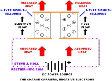
THE CHARGE CARRIERS, NEGATIVE ELECTRONS AND POSITIVE HOLES, TRANSPORT THE HEAT.
