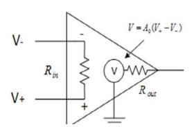
Open loop gain: It is the voltage gain of the op-amp when no feedback is Practically it is several thousands.
