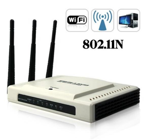
The **802.11n** standard can work over both the 2.4GHz and 5GHz bands, although most **802.11n** devices are restricted to the 2.4 GHz band only. ... Therefore, **802.11n routers** offer greater range and bandwidth than what is possible with the earlier 802.11g standard.
