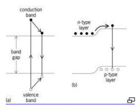
Recombination of electrons and holes generated by (a) optical absorption and (b) a forward-biased pn j unction
