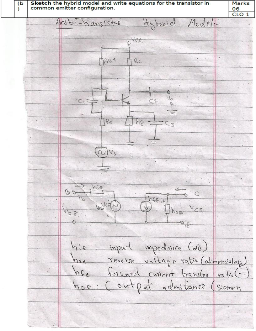
input voltage equation: Ube Voe = hipip + hye Vce Output wollage equation :- ic if ib is held constant (ib=0) then he & hoe can be solved hre = Vbe /uce 116 = 6 hoe = ic/Uce/16=0 Also of VCESS held emstant (VCF=a) than hie and hee can be solved: hie = Vbe/16/Vce=0. hee=fclib luce=0
