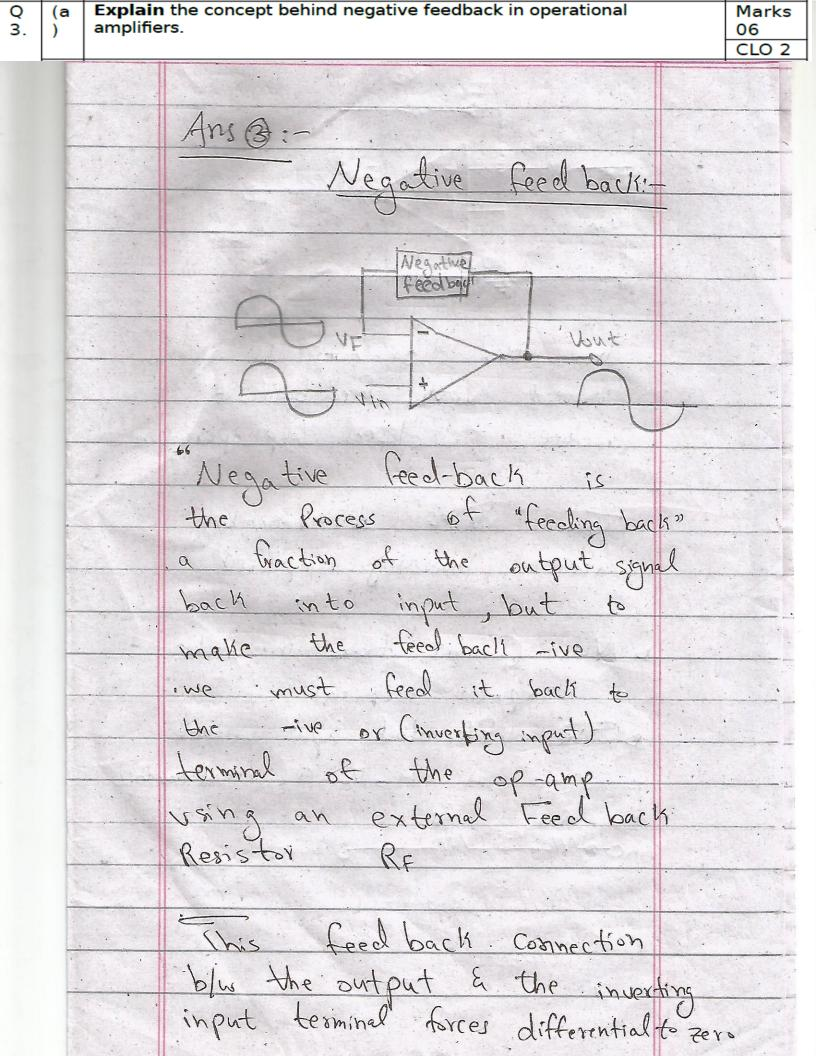
In this op-Amp is Connect with feed back to produce a closed loop operation Two rules to remember about Inverting amplifier DNo Current Hous into the input terminal is The differential Input voltage is Zero as V1 = V2 = O (virtual earth)
