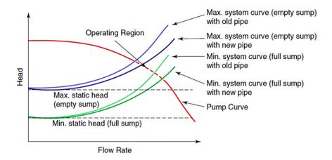
A system head curve is a common type of tool used in pump selection and system design and sizing. It combines elements of the performance (H-Q) curve of the specific pump under consideration with the combined static, operating, and frictional loss heads (The Total Dynamic Head Or TDH) of the system under design.
