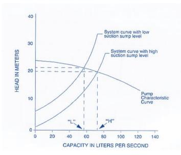
**Head** is the height to which a pump can raise water straight up. Water creates pressure or resistance, at predictable rates, so we can calculate head as the differential pressure that a pump has to overcome in order to raise the water. Normally expressed in Meters and Feet.
