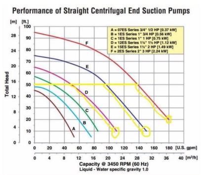
Situation #1: You are replacing an old pump that already has the pipes in place that are 2" going into the pump and 2" going out. The old pump is pumping water from a 5,000 gallon tank and pumping the water to a second tank that is 50 feet above the first tank. Your old pump was pumping approximately 100gpm (gallons per minute) and you would like to try to get a pump that will perhaps get you to 150gpm due to increased production demands.
