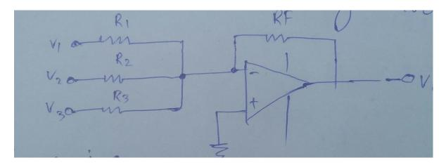
Summing amplifier is an application of inverting op-amp configuration that has two or more inputs and its output voltage is proportional to the negative of the algebraic sum of its input voltages
