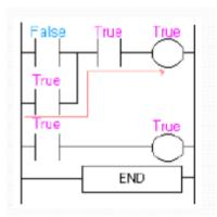
After scan 2 the oil level rises above the low level sensor and it becomes open. (i.e. FALSE)
