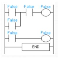
Since there is no more true logic path, output 0500 is no longer energized (TRUE) and therefore the motor turns off.
