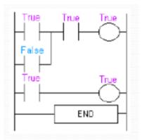
Initially the tank is empty. Therefore, input 0000 is TRUE and input 0001 is also True.
