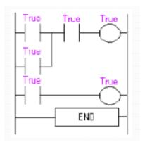
The internal relay is turned on as the water level rises.
