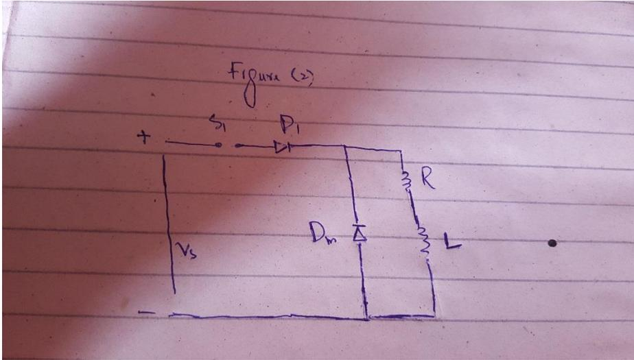
**When freewheeling diode is connected to RL circuit**
