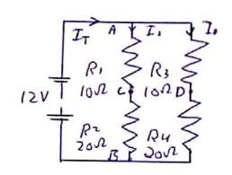
$V_{R_1}$ = 4V and  $V_{R_2}$  = 8V both Points have the same value of 8 voits; C=D=8 voits the difference is: 0 voits when this happens, both sides of the Parallel network are said to be balance because the voltage at Point C is the same value as the voltage at Point D. Qy. Ca)
