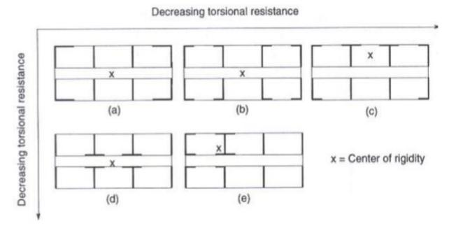
Greatest torsional resistance is obtained by concentrating the longitudinal walls at the comers of the building, as in Fig. a. The center of rigidity is at the center of the plan (from symmetry) and the longitudinal walls, being placed as distant as possible from this center, produce the greatest torsional resistance.
