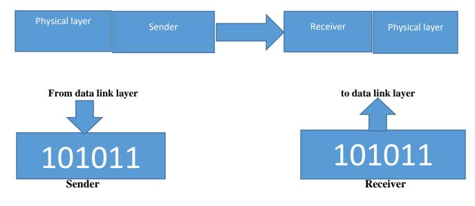
In the above diagram a physical layer provide functionality to data link layer all the data is passed from all the layers i-e (Data link layer, network layer, transport layer, session, presentation) and comes to physical layer for sending through transmission media.
