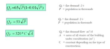
Total Storage Capacity = Balancing Storage + Breakdown Storage + Fire Storage
