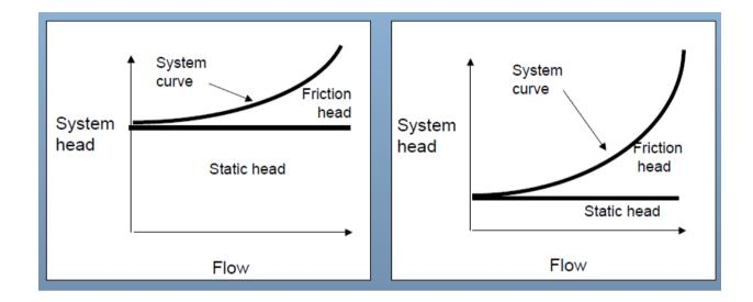
Static Head at any pressure is given as
