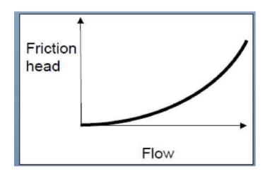
System Head is the sum of static head and friction head
