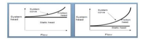
The formula for static head at any pressure is given by: Head (ft) = Pressure (psi) x 2.31/Specific Gravity
