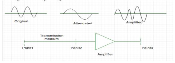
Attenuation is measured in **decibels (dB)**. It measures the relative strengths of two signals or one signal at two different point. Attenuation (dB) = 10log10 (P2/P1)
