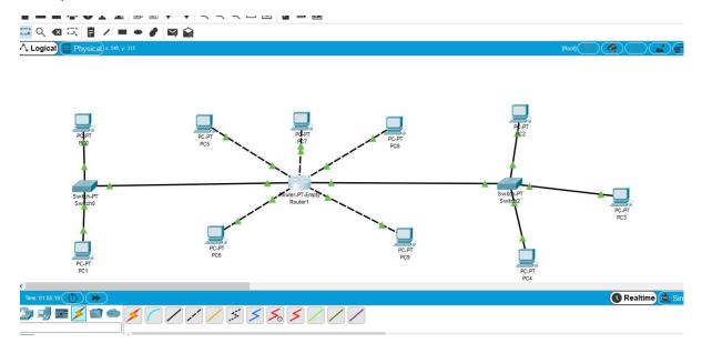
8. Assign the computers, switches and routers proper IP addresses, subnet mask and default gateways
