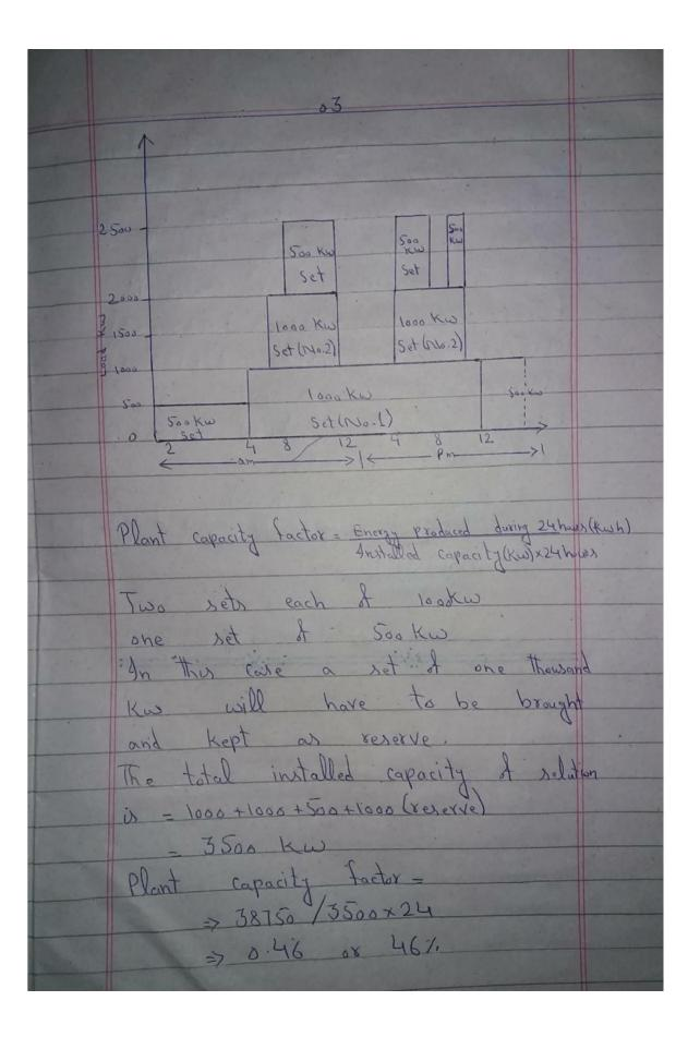
the operation sheduled fixed energy could have been generated by capacity of plant actually (500x6)+(1000x2)+(2000x2)+(2500x3) +(1500x1)+(2500x4)+(2000x2)+(2500x2 +(1000x2) = 39000 Kwh Energy actually produced = 38,750 Kwh Plant use 8.994 ox 99.4%
