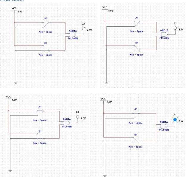
A dot (.) is used to show the AND operation i.e. A.B if A and B are the inputs to AND Gate.
